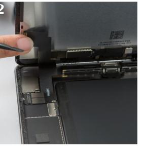
After the EMI shield is removed we can now disconnect the Digitizer/Lcd cables using the flat end of the spudger. Be gentle when disconnecting these cables. They are very sensitive so it's important not to break the pins. Take your spudger slide it underneath the cable flex the tool from left to right to disconnect such cables.
