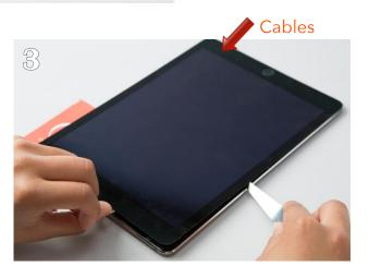
Tips: Taking your time throughout this process is essential and do not slide tool to far into the screen or you might scratch the lcd. If you can see the tool near lcd then you have gone to far into the glass with isesamo.
