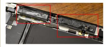
Tips: Put iPad on a flat surface!! Never start from the bottom the digitizer cable is located in that area as well as the home button significant pieces that should not be touched by metal.
