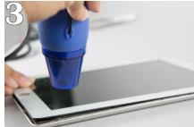
Tips: Taking your time throughout this process is essential and do not slide tool to far into the screen or you might scratch the lcd. If you can see the tool near lcd then you have gone to far into the glass with isesamo.
