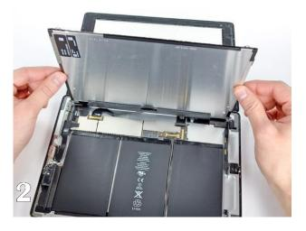
Tips: Try not to double up tape over same area will cause the screen to be lifted higher than normal.
