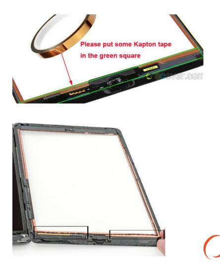
Tips: Try not to double up tape over same area will cause the screen to be lifted higher than normal.
